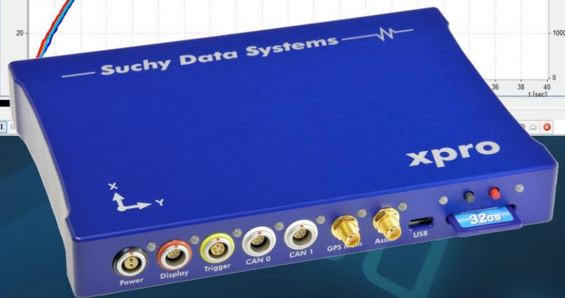
Top GPS, 4 CAN, 4 Zähler, 4 Analog-In, Altimeter, Inertial Sensor
